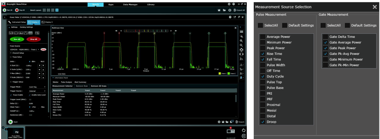
Figure 9. Multi-channel trace display with 4-pairs of gates and automatic pulse parameters measurement (sample screen shot with two U2042XAs).
