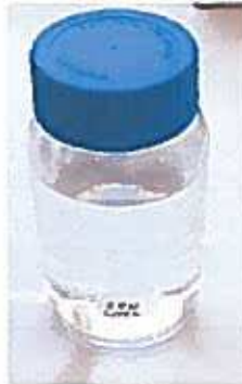
Figure 5: Example of acceptable 1 liter glass bottle for particle and NVR level rinse validation.
