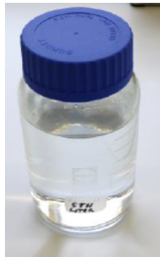
Figure 4: Example of acceptable 1 liter glass bottle for particle and NVR level rinse validation.
