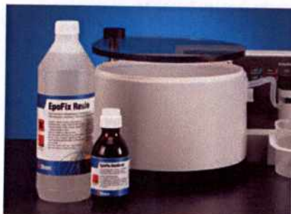
CitoVac with Struers impregnation material (EpoFix)
