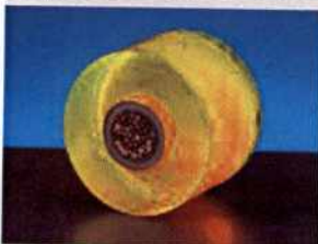
Cable mounted with EpoFix and EpoDye.
