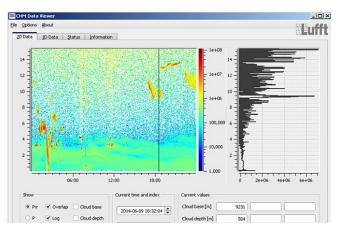
The CHM Data Viewer is a special visualization software with an easy to use interface. The software allows a representation of the data, which are measured with the Laserceilometer CHM 15k. The data is previously stored as raw data in NetCDF format and can be visualized and saved as an image file with the Data Viewer.
