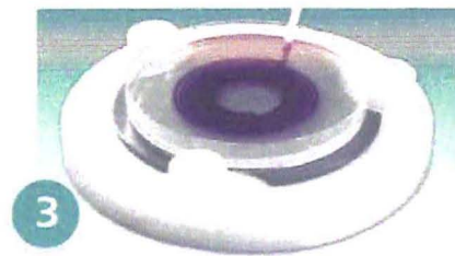
As the agar plate spins, the syringe automatically dispenses accurate volumes of sample over the plate drawing a spiral with the loaded sample
