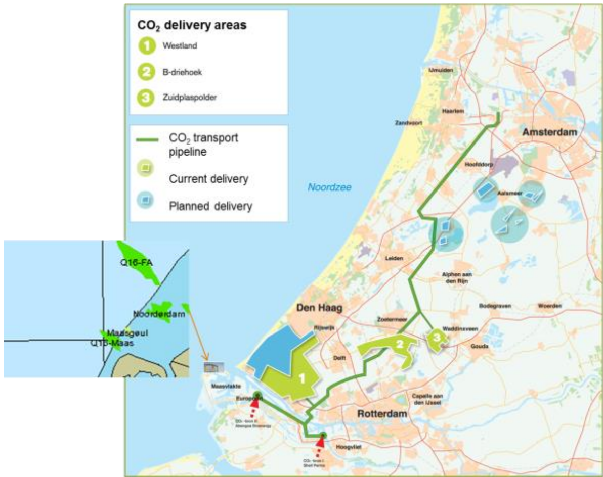
Schematic of the existing infrastructure for delivery of CO 2 to the greenhouses and the planned additional infrastructure including the CO 2 buffer
