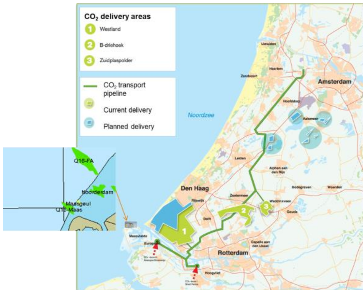
Schematic of the existing infrastructure for delivery of CO 2 to the greenhouses and the planned additional infrastructure including the CO 2 buffer
