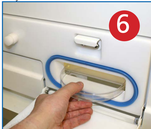
9cm Front Loading or 15cm Side Entry Letterbox - Ideal for introducing individual samples quickly.
