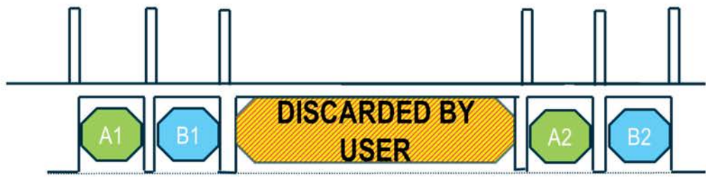
Figure 6d: Paired sequence with long delays between paired images. In this case a set of images is required with a long delay between their capture. This would require an extra exposure to be taken and the image discarded by the user.
