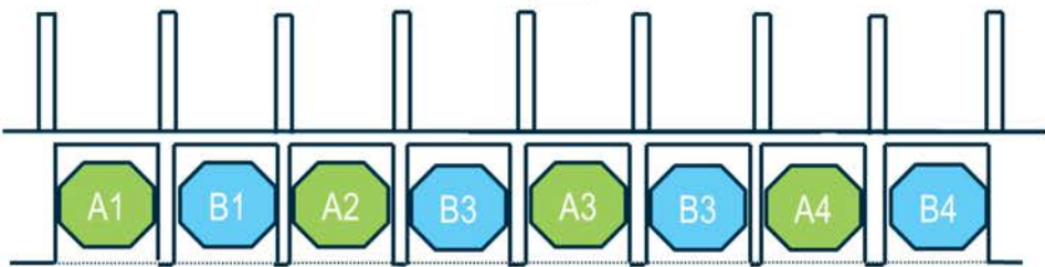
Figure 6c: Long sequence of paired PIV images. The images do not need to be single pairs but can be setup in long sequences. The exposure time can be varied image to image if required.
