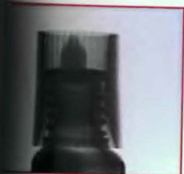
Sample is too far away from the X-ray source, low magnification
