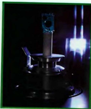
For highest resolution rely on the integrated micro-positioning stage and insert the sample manually
