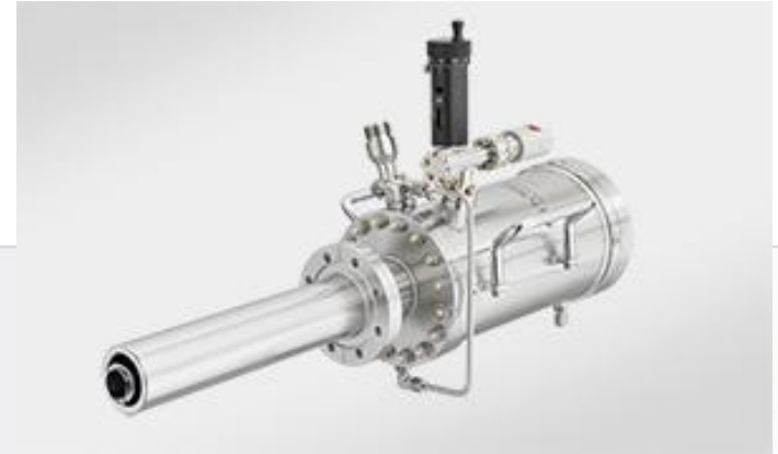
VACS 100-300 valved arsenic cracker with DN63CF (O.D. 4.5") mounting flange (using a VADP 100-63 adapter), 300 cm 3 crucible, cooling shroud and motor drive
