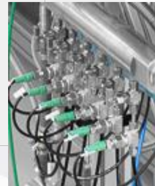
Water panel with individual flux sensors
