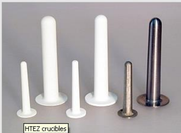
Crucibles for HTEZ made of \text{Al}_2\text{O}_3 , BeO and refractory metals (W, Ta), sizes 1.5 and 10 cm 3
