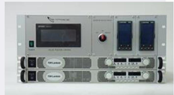
Motorized Valve Control Unit and DC power supplies
