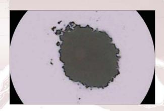
The CCD image above shows an example of a small sample analysis. The sample (the dark center measuring approximately 11 mm) was imbedded into boric acid and pressed into a 30 mm pressed pellet. Utilizing Micro Analysis, a 10 mm analysis can be performed on the sample area, eliminating the surrounding boric acid from the calculations.
