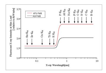
Enhanced sensitivity from 30  $\mu$  tube for enhanced light element analysis.
