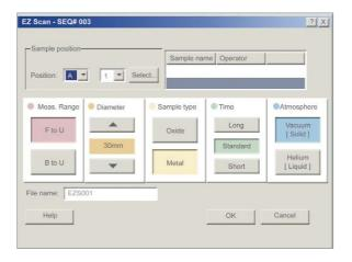
EZ Scan provides quick Semi-quantitative set-up to determine intensities.
