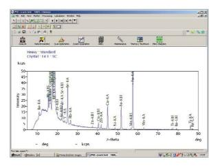
SQX data treatment uses FP-based software to calculate unknown concentrations.
