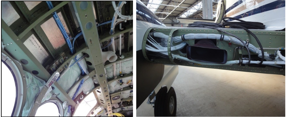
Figure 3.18: Examples of Wiring Harness Installations
