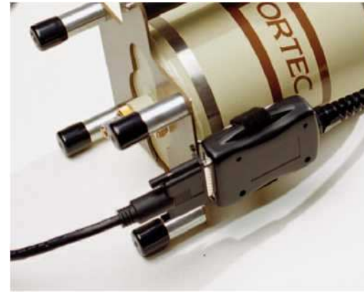
SMART-1 Detector Interface Module.
