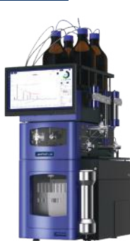
puriFlash® 5.250 250 mL/min - 250 bar Optimized for your preparative purifications
