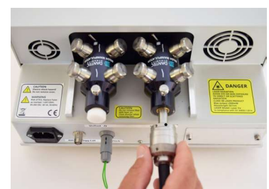
Laser light is shut off when the fiber plug is removed
