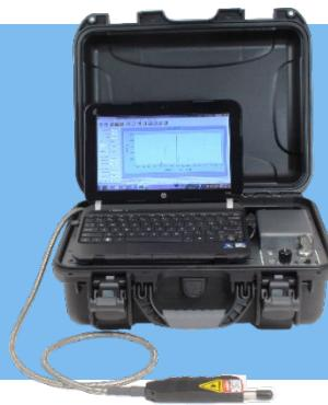
The PolyLab Plastics Analyzer system features a narrow linewidth frequency stabilized laser, high throughput fiber optics probe, and an optically fast (f/1.6) spectrograph with TE cooled CCD detector. This system is easy to use with powerful and user-friendly RamanReader software, while providing excellent long term reliability with minimal maintenance.
