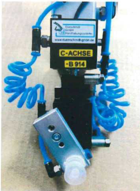
C-axis: 6 tap holes M5 for fastening the gripper
