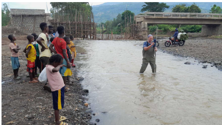
Example of discharge measurement with OTT MF Pro in Gofa zone.
