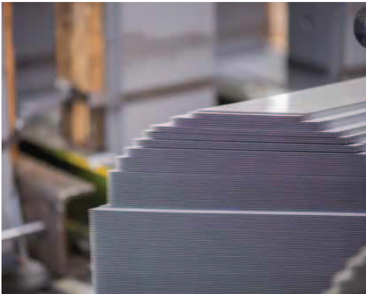
Step-lap technique permits ideal energy flux within the core
