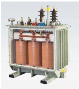
Distribution transformer with extremely low losses thanks to amorphous core material
