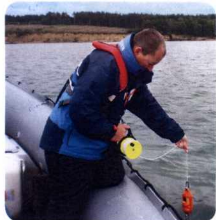
The CastAway incorporates the most modern technology available yet is simple to use. It is designed for profiling down to 100 m and is easy to deploy.
