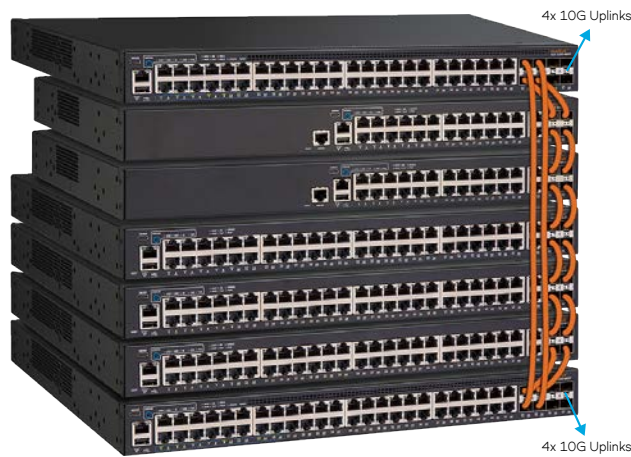
Figure 1: Up to 12 RUCKUS ICX 7150 Switches can be stacked together using up to four SFP+ 10 Gbps ports per switch for a fully redundant backplane delivering 480 Gbps of aggregated stacking bandwidth.
