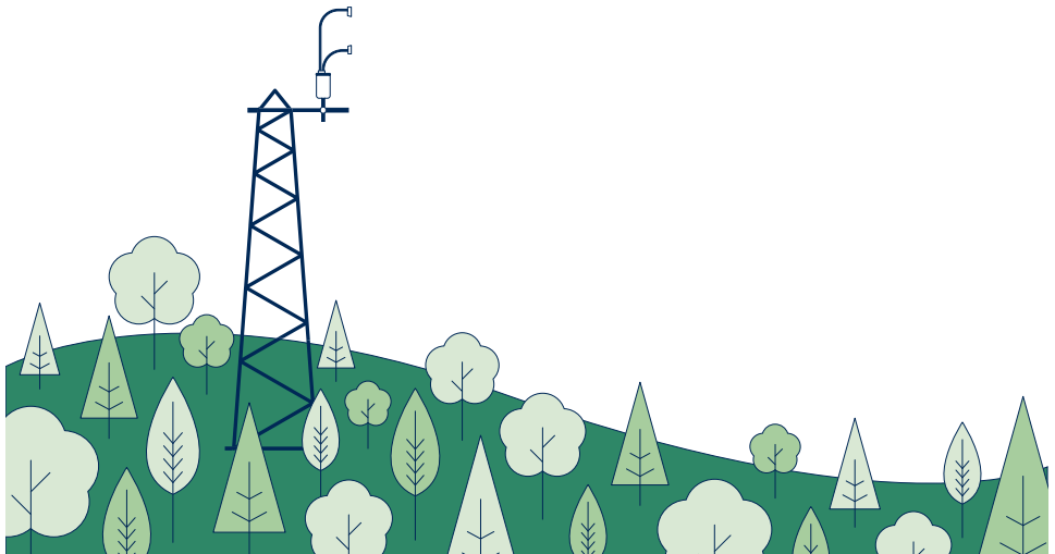
Figure 2-7. The LI-710 should be at least 2 meters above the top of orchards, woodland, and forest canopies.
