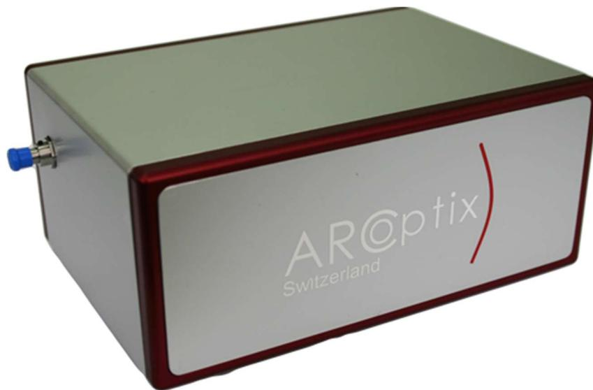
Figure 1-1 The Fourier-transform spectrometer FT-NIR Rocket. One distinguishes the input connector for the optical fiber, bringing the light into the spectrometer. Data transfer to the computer and power supply (for non-cooled detectors) are done by the USB connection.
