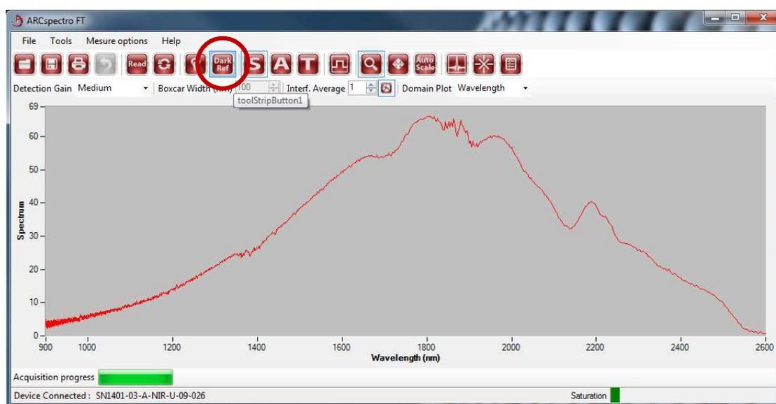
Figure 3 - Dark signal measured with an internally illuminated integration sphere
