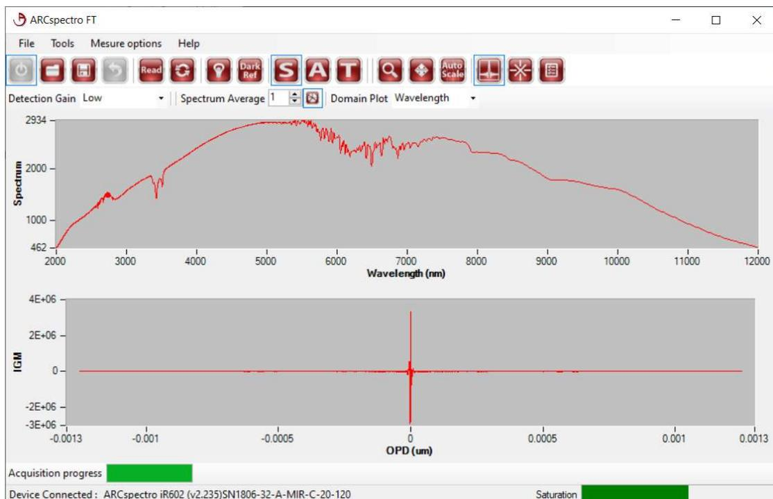
Figure 4-1 - Spectrum and corresponding interferogram (IGM)
