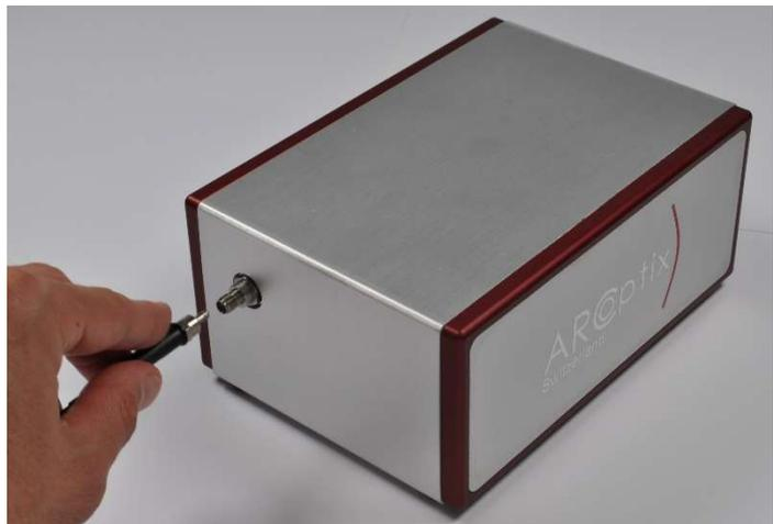
On the FT-IR 2-12 (and some customized systems), the fiber coupler is external and removable. This is useful if you want to couple a free-space propagating beam into the spectrometer.
