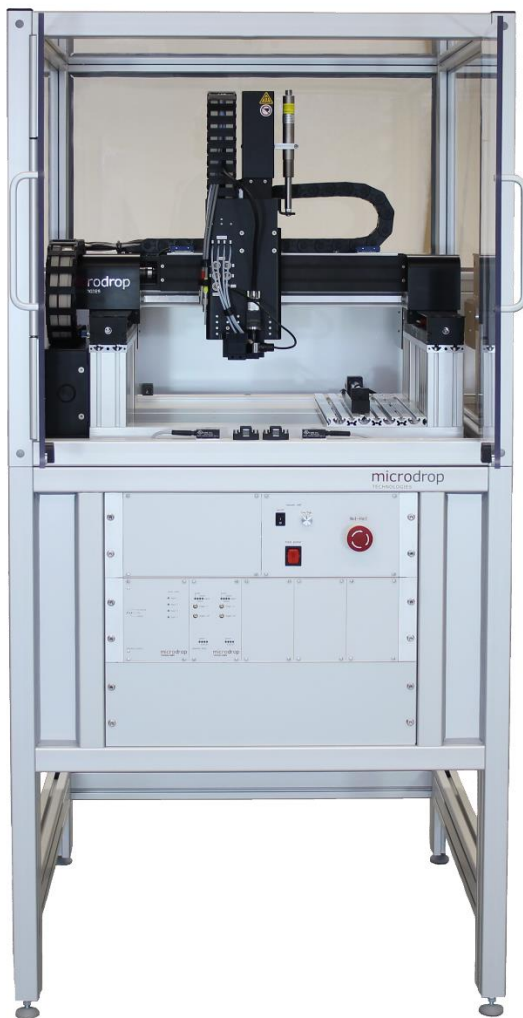
Figure 2: Autodrop Gantry II Printing System, here with underframe and hood
