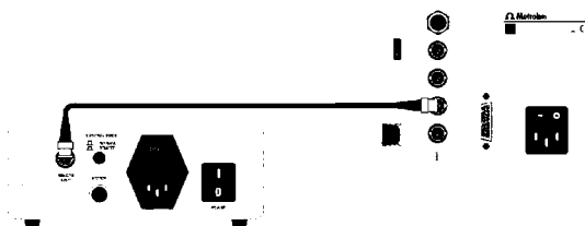
Figure 45 Connection between the Remote Input of the Motor Controller (left) and the Analog Output (A-OUT1) of VIONIC (right) using a BNC cable.
