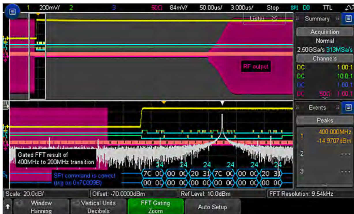
Figure 21. Triggered on a SPI command, the RF signal is still at 400 MHz as indicated in the frequency peak search result list.
