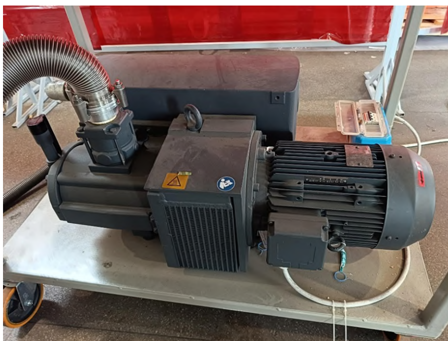
Fig. 3 Rotary pump (Pompa rotative)
