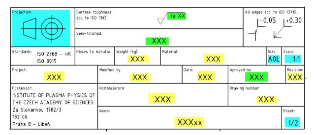
Every drawing shall include the main drawing title block with all essential information about a part or assembly as shown in figure above. All coloured fields have to be filled individually according to the naming convention and CAD model. In case any field should stay blank use "---".
