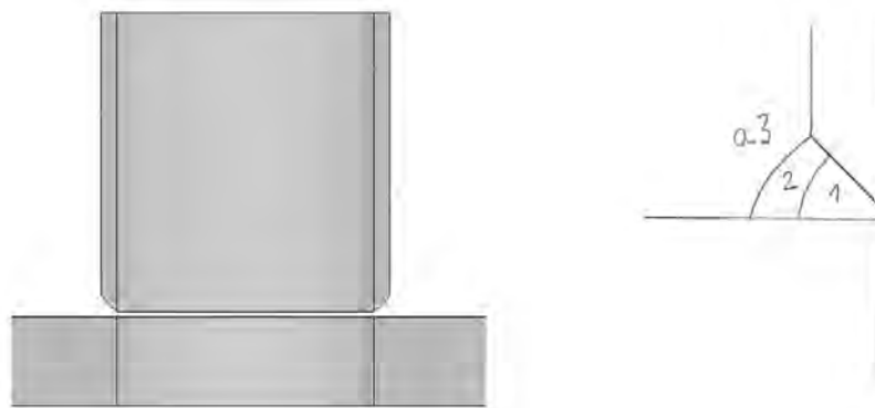
Figure 2.30 – Preparation of weld bevel and corresponding schematics of weld passes layout for joint of the vertical port shell to the VV wall
