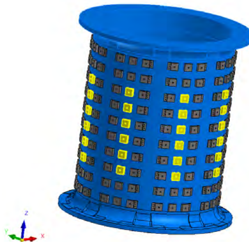
Figure 4.2 – HFS-middle adapters, six rows around the meridian line
