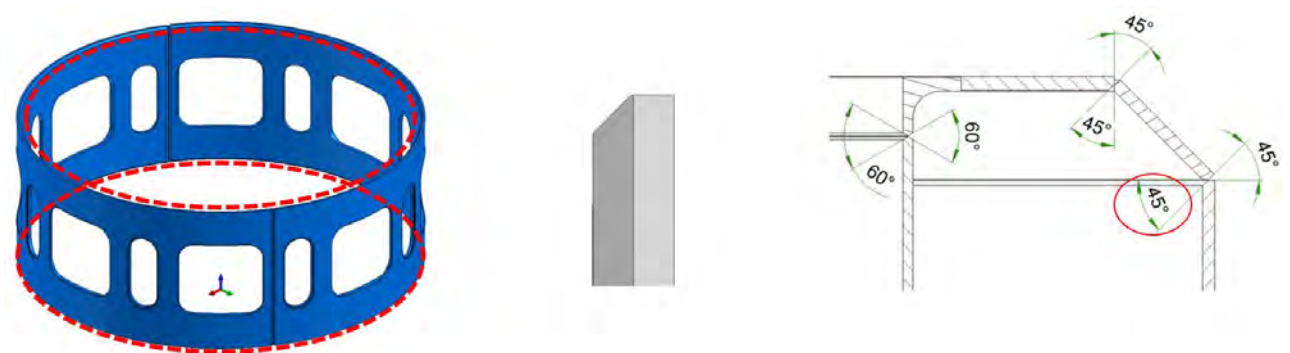
Figure 2.22 – Bevel preparation for the welds to cones
