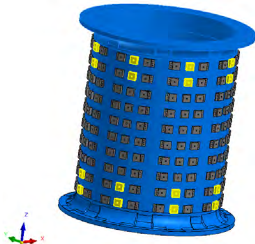
Figure 4.4 – HFS-middle adapters, two upper and lower rows
