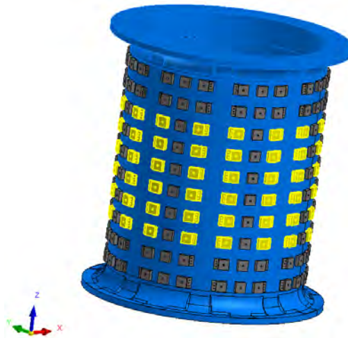
Figure 4.5 – HFS-side adapters, six rows around the meridian line
