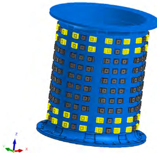
Figure 4.7 – HFS-side adapters, two upper and lower rows
