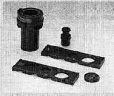
ELWD Condenser and phase sliders
