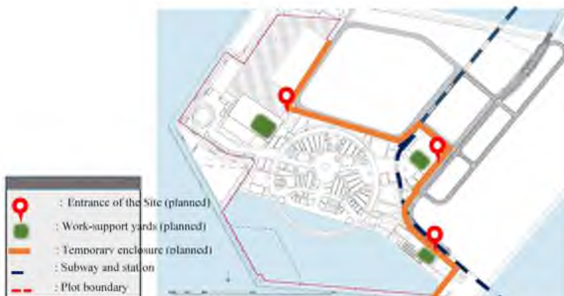
Figure 5.2 Draft Installation Plan for Temporary Construction Facilities in the Site (Planned)
