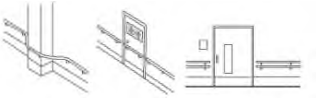
Figure 3.18.1 Handrails (illustration of continuous handrails)
