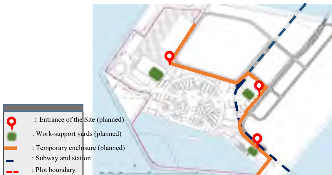
Figure 2.2 Draft Installation Plan for Temporary Construction Facilities in the Site (Planned)
