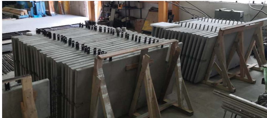
• Fig. 2 – Battery of thin concrete composite-reinforced panels ready for assembly
