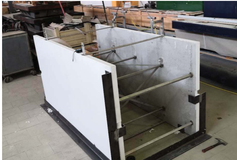
Fig. 4 – assembled prefabricated segment in assembly stand
