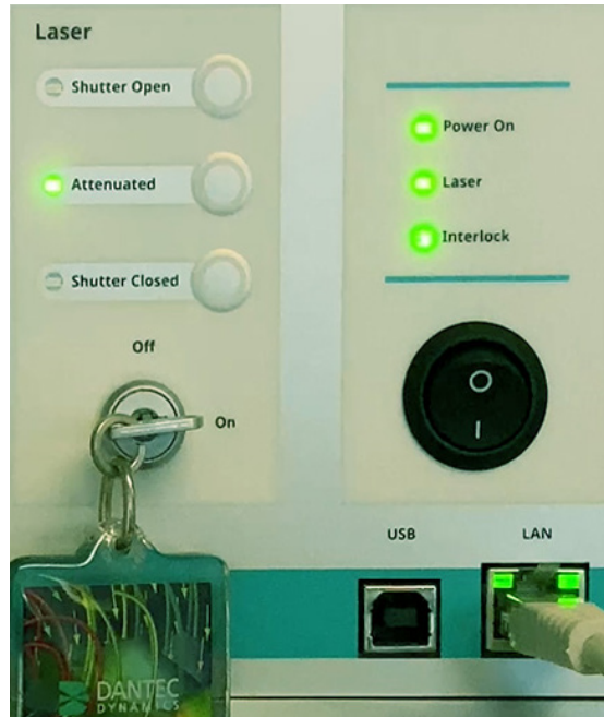
Laser controls, status lamps and interfaces on the front panel
