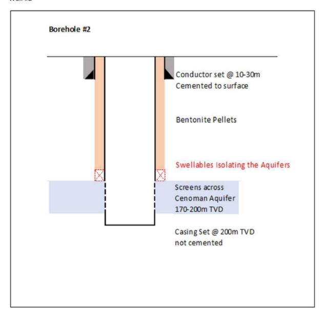
Figure 4 Diagram of Well #2
