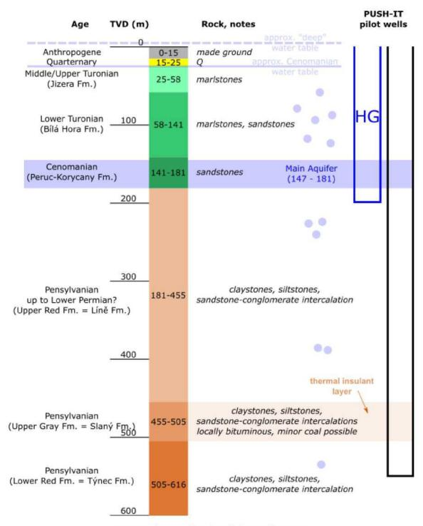
Figure 1 Relevant geological Profile from Well GTPVLT-1
