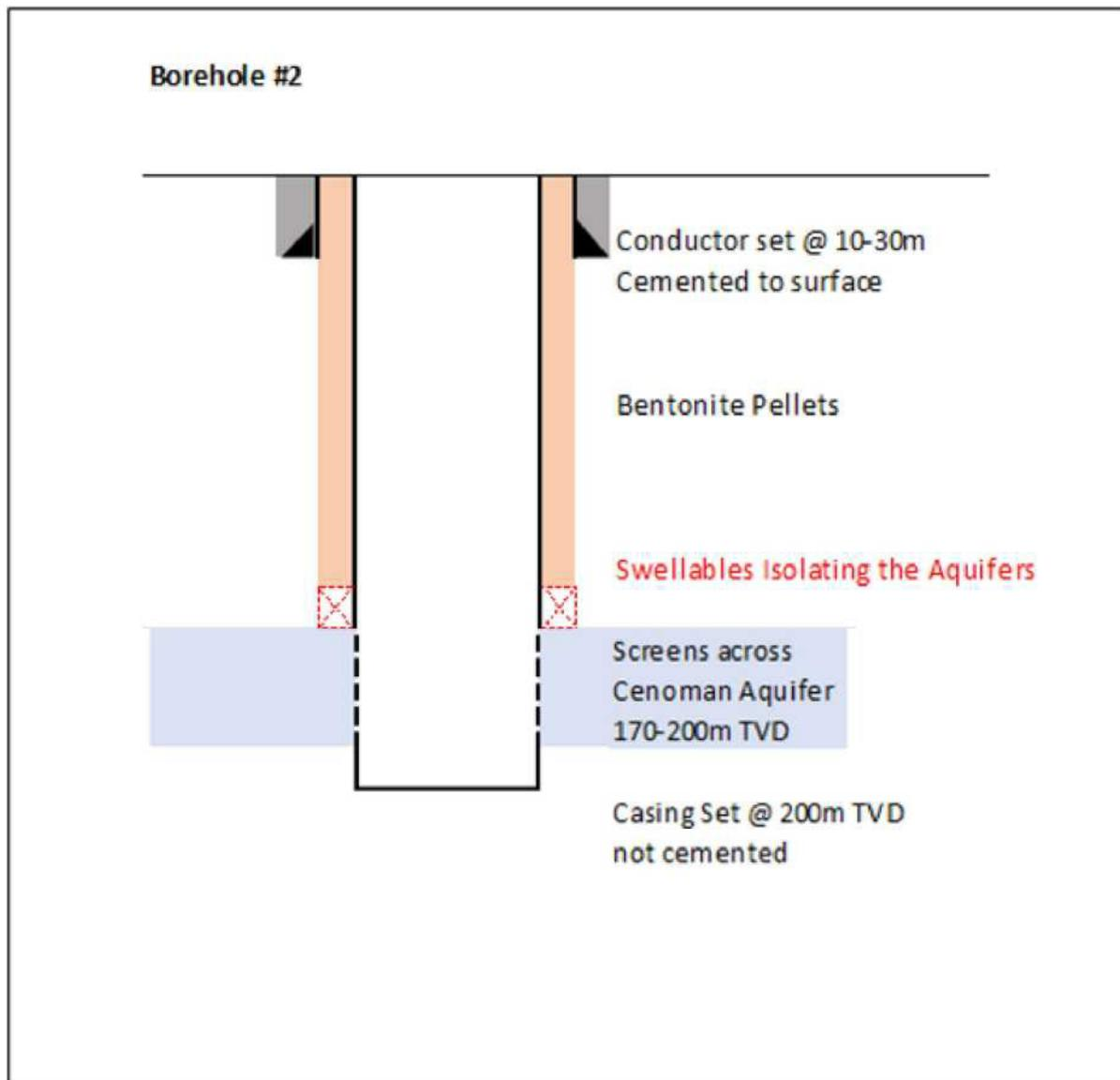
Figure 4 Diagram of Well #2
