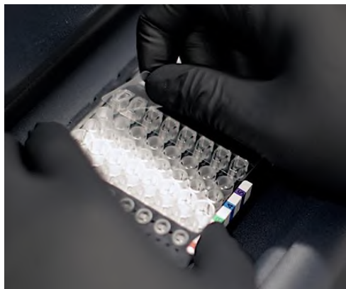
Figure 6. Remove the plastic film from the sample wells.
