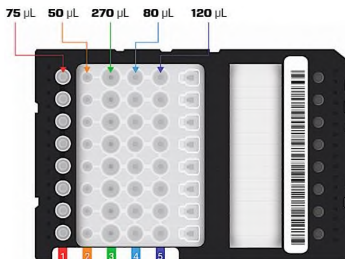
Figure 5. G2 FFPE To DNA purification buffer dispense volumes.
