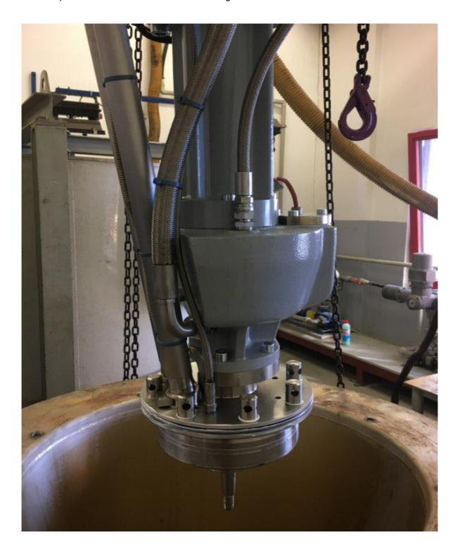
By hand is tested the oil circulation, all was working. The signals and vibrations will be tested during the test in the absorber.
