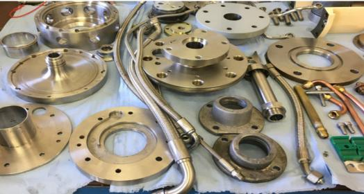
The complete atomizer was built up with new gaskets and O-Rings.
