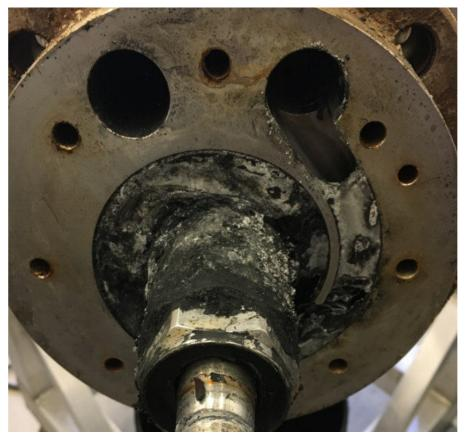
The next step was to check the feed inlet on the extension part of the main motor, here we see that someone changed the inlet from the left (lower volute) to the right side (upper volute)
