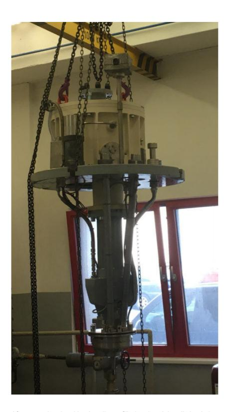
After mounting the skirt, the oil was filled up hand the oil circulation was tested by hand.
