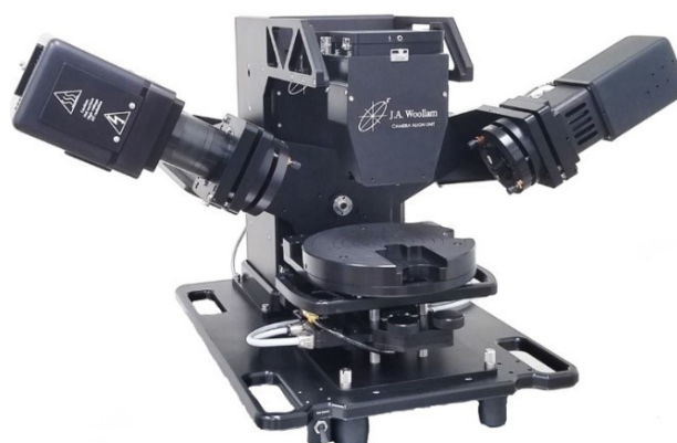
M-2000 with automated angle base, featuring a horizontal sample mount.
