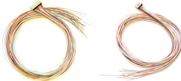
Figure 9. 36-pin wire adapter for 32-channel stim/record headstage (left). 18-pin wire adapter for 16-channel headstage (right).
