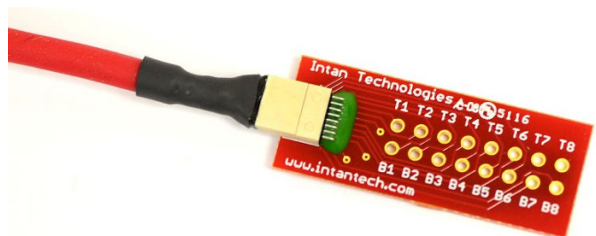
Figure 11. Stim SPI cable adapter board plugged into RHS Stim SPI interface cable.
