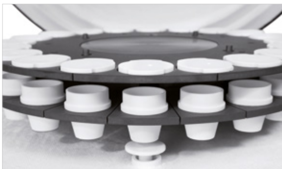
PC-controlled application of crucible lids / crucibles open
