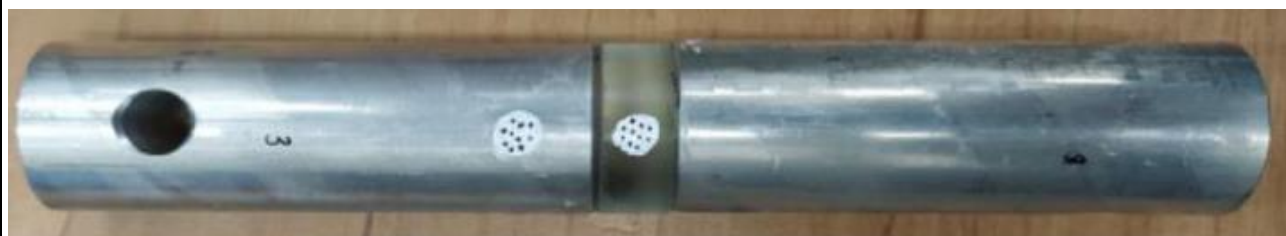
Figure 1: Tensile coupons test setup: Aluminum rod (Al6061) vs. 0.5mm 93-500 DS vs. glass/crystal-epoxy glue vs. aluminum (not specified) rod
