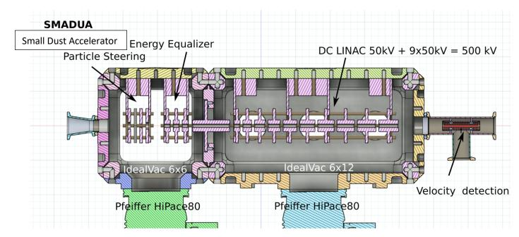
Electrodes: Stainless Steel Isolators, holders, screws, etc: PEEK
