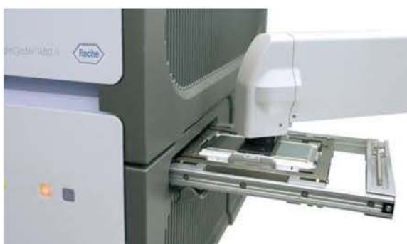
Figure 19: Automated LightCycler® 480 Instrument loading process.
