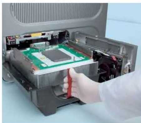
Figure 1: Flexibility of the LightCycler® 480 Block Cycler unit. The LightCycler® 480 Block Cycler units (96-well/ 384-well format) are easily interchangeable by the user, taking only a few minutes. The exchanged block cycler unit is automatically detected and identified by the system, and experiments can proceed without time-consuming recalibration runs.
