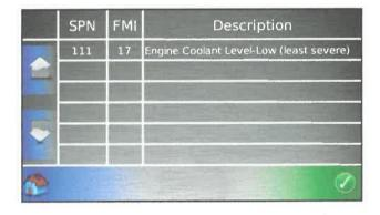
Engine diagnostic via J1939 CAN bus protocol
