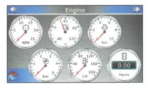
Dedicated parameters display is also available for the technician during maintenance in order to check signals from various sensors and activated inputs/outputs.
