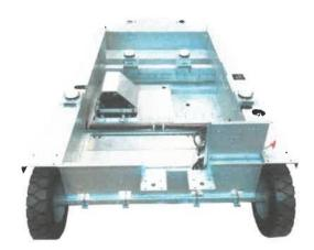
A large storage compartment is fitted on the front side of the chassis, allowing easy storage of the air delivery hose(s).
