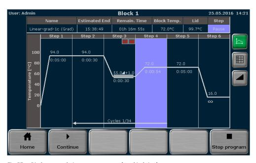
Fig. 57 Display screen during a program pause (graphical view)
