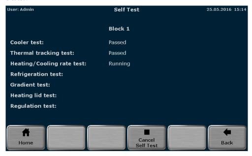
Fig. 97 Extended self-test overview screen (Biometra TAdvanced Mono)
