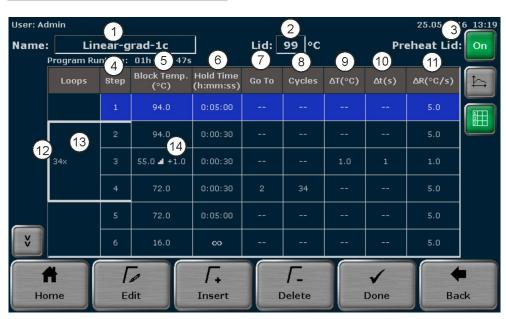
Fig. 22 Spreadsheet programming
