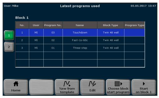
Fig. 16 Program quick start screen (Biometra TAdvanced Twin)
