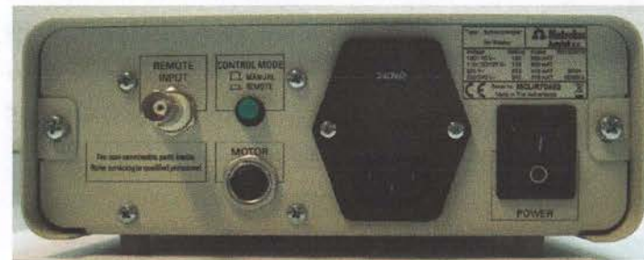
Figure 4 – Motor controller (back plane)
