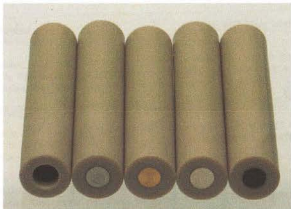
Figure 2 – Overview of the 5 mm tips compatible with the Autolab RDE
