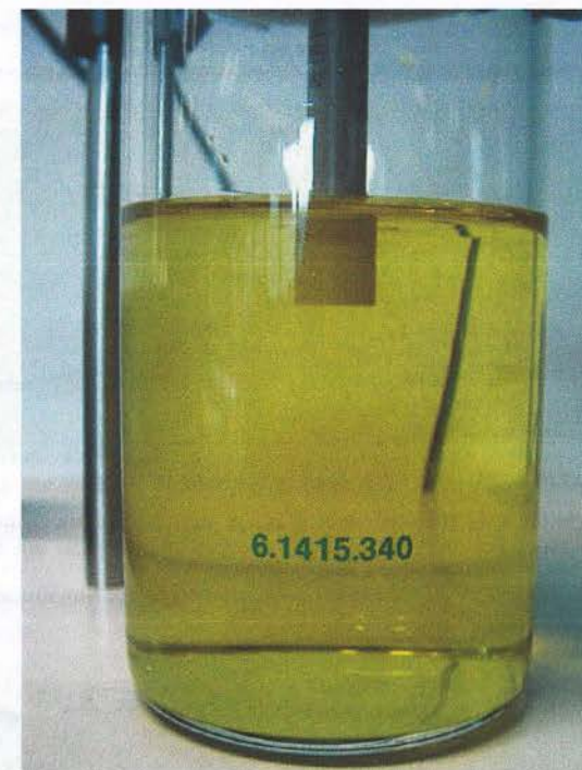
Figure 7 – Correct position of the RDE in the cell
