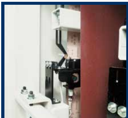
Belt oscillation controlled by an electronic photocell for longer life span of the belt.
