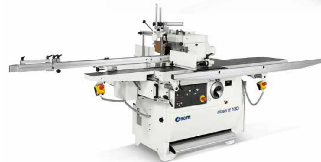
"TL" versions Top machining precision and stability due to the manual feed carriage with castiron structure mounted on axial bearings running on slideways made from hardened and ground bar.
