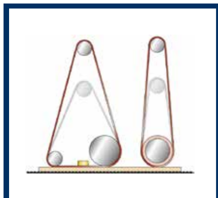
Long belts: 2620 mm length for greater productivity and less downtime.
