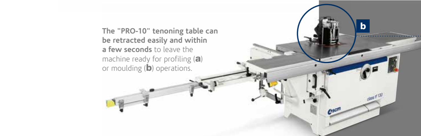
"TL PRO-10" versions The manual feed carriage is a cast iron structure running on linear slideways with recirculating ball screws, guaranteeing maximum machining precision and stability.
